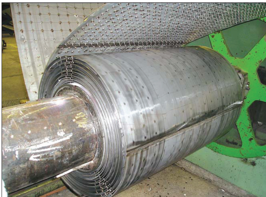
Figure 1 Production of the SHE heat-transfer body
